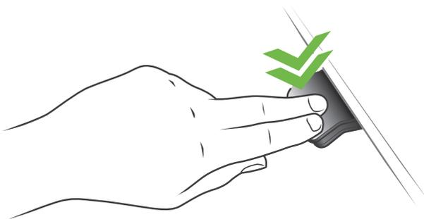
Figure 34: Double tap to adjust the desk to a memory position automatically
