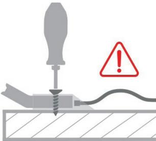
The screws must be fastened sufficiently, but without damaging the plastic.
