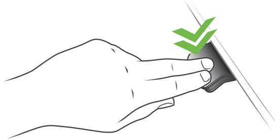
Figure 24: Double-tap to automatically adjust the desk to a favourite position
